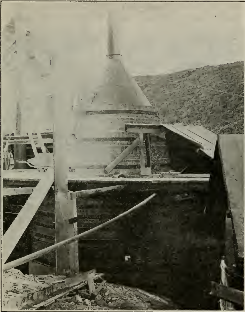
Shaft furnace of Western Magnesite Development Co., at Red Mountain, Santa Clara County, California.
